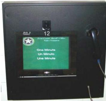
All MRF series enclosures are constructed of 14-gauge steel with a heavy duty, more resistant 3/8" thick polycarbonate window. MRF enclosures are heavy-duty powder coated for durability and ease of maintenance. Welded steel panels and rugged construction protect equipment from being damaged in environments subject to heavy use and abuse. The viewing area behind the polycarbonate window is 12" H x 15" W.
