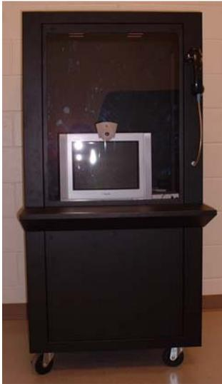
Strike's Mobile Visitation Station is specifically built for the corrections environment. The unit is black powder coated, constructed of 14-gauge steel and has a large polycarbonate window that can be left clear or masked to match the size of the viewing opening to the size of the equipment selected. The unit has heavy-duty locking casters for easy mobility allowing it to be moved from one area to another and then locked in place when in use or placed in storage.
